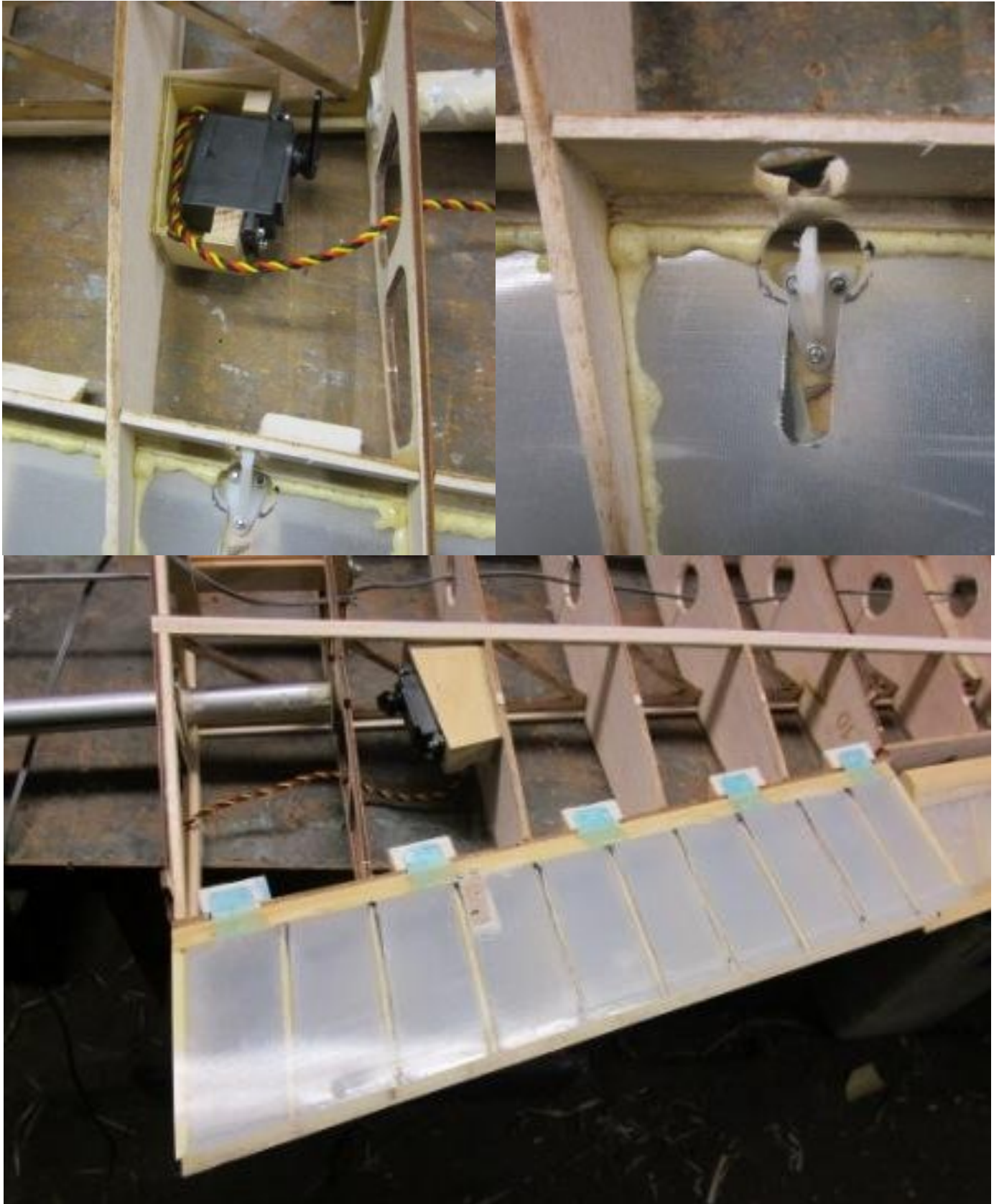
The top left picture is of the angled servo box glued to a rib and the rear spar. The back of the balsa rib will be reinforced with a spruce bearer. The top right picture is of the keyhole in the floor of the flap recess and of the simple commercial horn attached to the leading edge of the flap. The bottom picture is of the build up on the front of the flap recess to take the five strip hinges.
